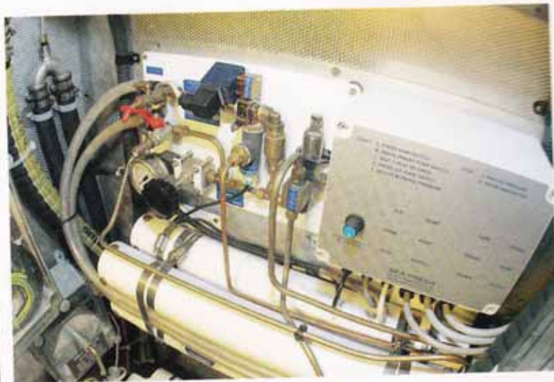
Left: adding biocide 'pickling' is easy. It takes a couple of minutes and preserves the membranes for up to 12 months
