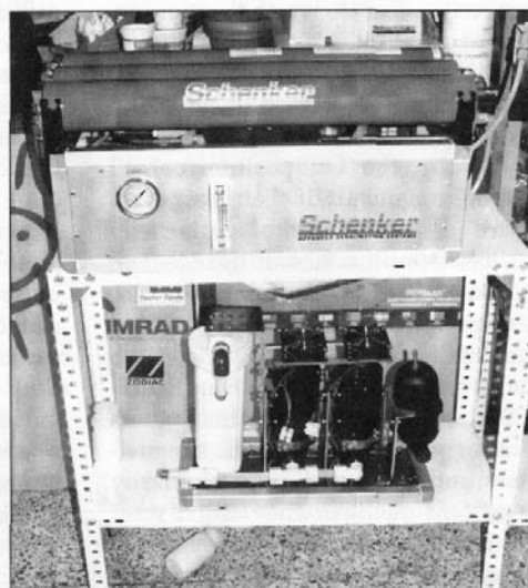
Above: Schenker's largest watermaker uses dual low-pressure pumps (bottom) and three standard 2521 membranes. Below: Smaller models use two membranes plus single or dual pumps.
