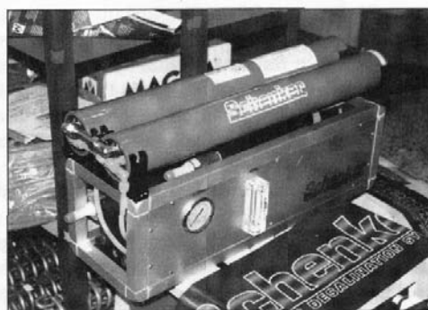
Above: Schenker's largest watermaker uses dual low-pressure pumps (bottom) and three standard 2521 membranes. Below: Smaller models use two membranes plus single or dual pumps.
